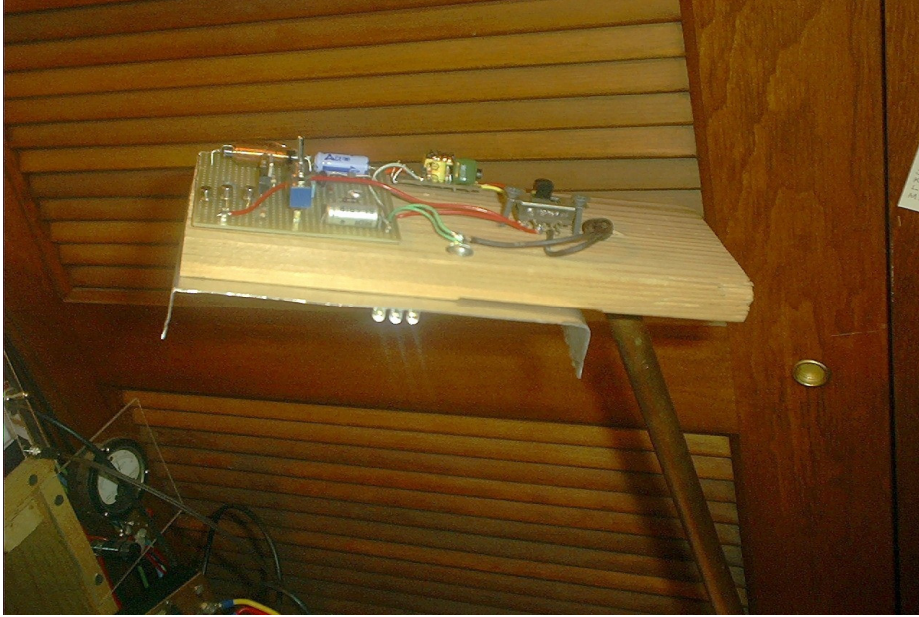
A homebrew LED and fluorescent station lamp
