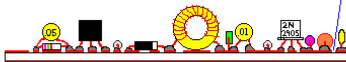
"Gouged Board" - Parts soldered to islands and traces on 2-sided p.c. board.
