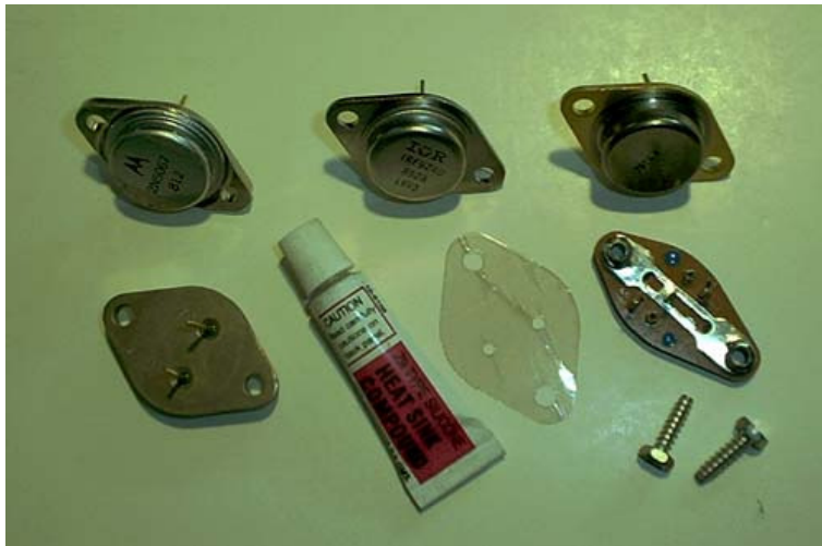
Power bipolar and MOSFET transistors and the necessary size TO-204 mounting kit
