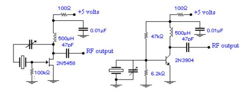
Two common crystal oscillator circuits
