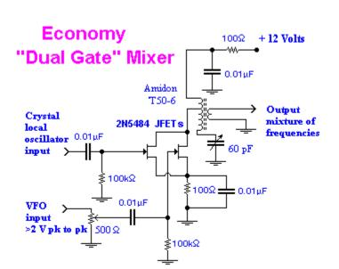
NTE-222 and NTE454. This application is quite uncritical and I believe any dual gate will work well. You will find that mixers in superhetrodyne receivers are not so uncritical.
