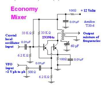
both input signals are small, both transistors will need forward bias, the 33K resistors. If one of the inputs is large enough, say 5 volts peak or larger, you won't need the forward bias for that input. This circuit should be plenty sensitive for a receiver mixer. However, because it has PN junctions, it will be noisier than the dual–gate MOSFET mixer and I don't recommend it for receivers.
