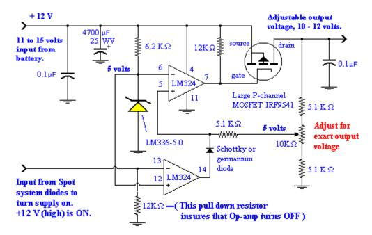
Low Dropout 12 Volt Power Supply with Remote
