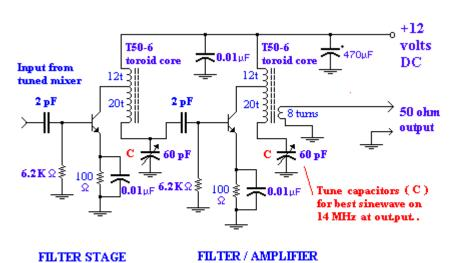
FILTER FOR 20 METER CW (14 MHz)
