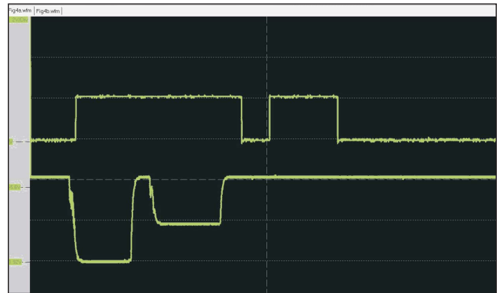
Figure 8—Lower trace, KEYIN; upper trace, transmitter control. C6 has been increased to almost 0.1 uF.
