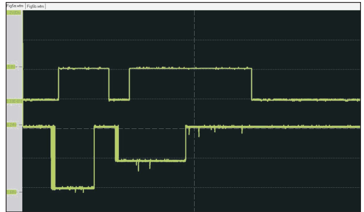
Figure 10—Lower trace, KEYIN; upper trace, transmitter control. C6 has been reduced to 100 pF.
